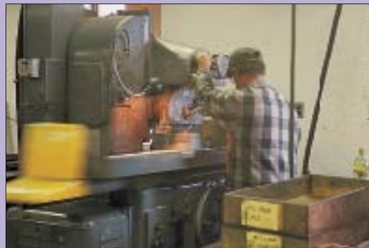
After rough milling the plane bodies are ground to make plane sides smooth and square
