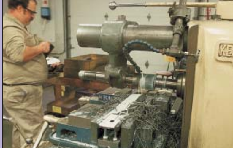
The bottom of the iron plane body is milled flat and true
