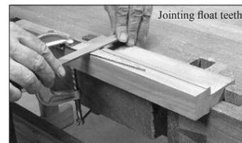
Sharpening floats is much like sharpening hand saws; jointing is necessary after the first few sharpenings to maintain even tooth height. Joint teeth by draw filing with a 6"-10" single cut mill bastard file. Hold the file at a right angle to the float's edge and lightly push the file forward. All that's needed is to create the slightest flat on each tooth, which brings them to the same level.
