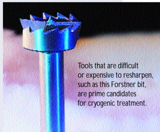
Tools that are difficult or expensive to resharpen, such as this Forstner bit, are prime candidates for cryogenic treatment.
