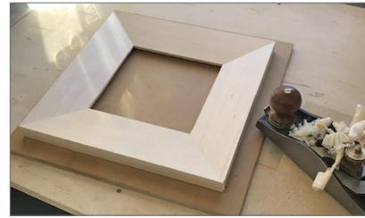
In this workshop, furniture maker and educator Mason McBrien will show students techniques for cutting, trimming, and assembling accurate mitered frames by hand. Students will practice cutting and truing miters to an accurate 45° angle, laying out and trimming frames, and cutting rabbets for inset wood, glass, or mirrors—all using traditional methods of hand work which are safe, quiet, and precise.
