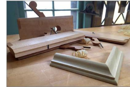
This class will focus on creating various moldings using hollows and rounds sized 6 and 10 along with a rabbet plane. From layout to execution, ranging from simple coves and ovolos through ogees, cymas and various combinations. Each
