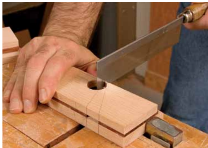
Big hole helps clear shavings. Use a Forstner bit at the drill press to cut a hole that meets the bed but does not cut into it. To help the chips reach the hole, saw a slot that lines up with the mouth.
