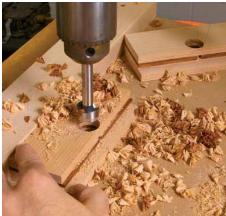
Big hole helps clear shavings. Use a Forstner bit at the drill press to cut a hole that meets the bed but does not cut into it. To help the chips reach the hole, saw a slot that lines up with the mouth.
