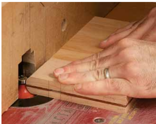
Big hole helps clear shavings. Use a Forstner bit at the drill press to cut a hole that meets the bed but does not cut into it. To help the chips reach the hole, saw a slot that lines up with the mouth.
