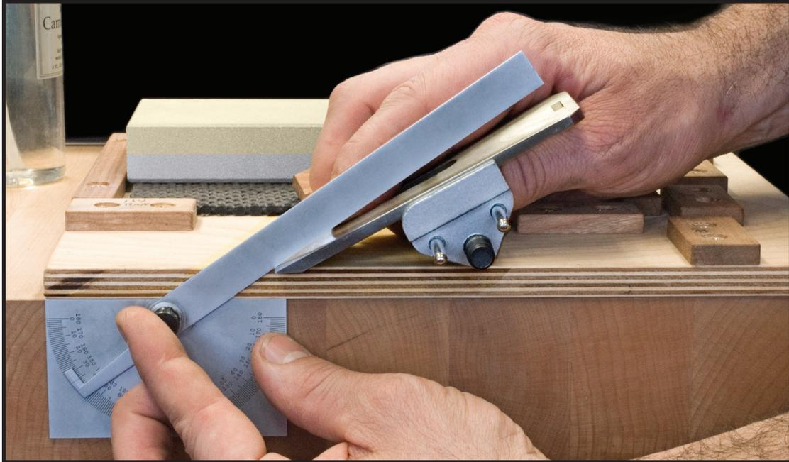
Adjust the position of the blade to match the angle of the protractor arm. The resulting projection distance gives you the position for the stop.
