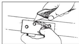
2. Now you're ready to set the blade of your Butt Mortise Plane, using the leaf of your hinge. We recommend that, on your first several mortises, that you not set the plane to the full depth. Start with a healthy cut, though — at least half the depth of the finished mortise.
