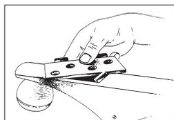
3. The final step is to plane out the area to be mortised. Start on the outside or open edge. Work the length of the hinge in both directions and with overlapping cuts until you have a perfectly square and smooth mortise.
