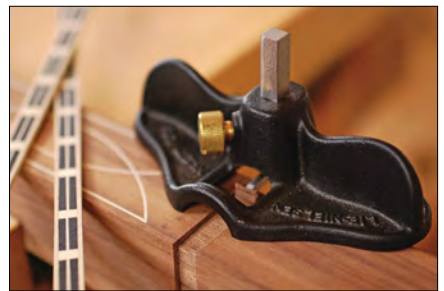
Three specialty blades designed for inlay work: ⅜" square tip ¼" pointed tip ⅜" pointed tip
