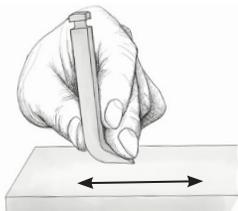
1. First, hone the bottom of the blade. Make several passes along a waterstone until a slight burr is formed along the cutting edge.
