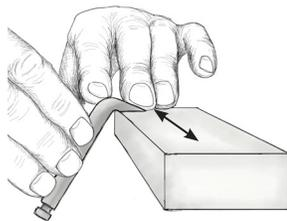
2. Then flip the blade over and make a few light passes along the beveled face to remove the burr and polish the bevel.
